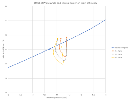
Figure 19: Control phase swept for 3 different alpha ratios at a fixed BPA input power.
