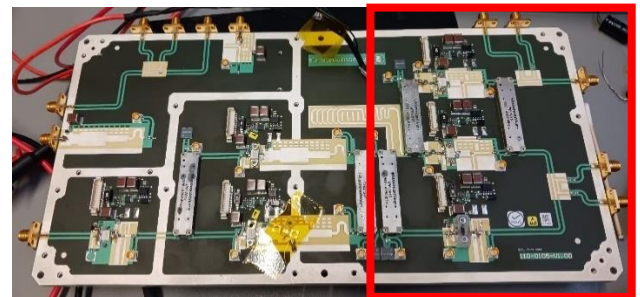
Figure 18: Full Prototype LMBA hardware PCB Assembly, mid-development. LMBA configuration can be seen in the red box.
